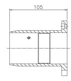
PART No. T20289 THREAD M56x1.5mm PITCH ISO 4 HOLES Ø5.4 CBORED Ø9.4x5.3 DEEP EQUISPACED ON 80 PCD
