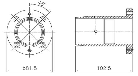
PART No. T20096/B THREAD M45x1.5mm PITCH ISO QUICKLOCK STYLE FLANGE
