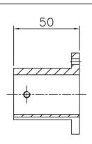
PART No. T21461 4 HOLES Ø4.5 POSITIONED AS SHOWN ON 50 PCD
