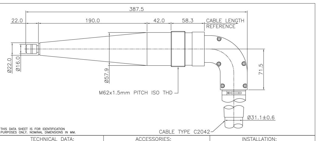
TERMINATION:-CLAMPING SLEEVES:-WARNING: NOMINAL OPERATING VOLTAGE 210KV DC STANDARD FLANGE T20172/A CABLE SHOULD ONLY BE FITTED BY A TRAINED PERSON.
